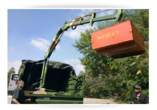
Regiment of Artillery is in the process of modernising its capabilities. All future medium guns are planned to be 155 mm/39/45/52 Cal, thus, ensuring common 155 mm ammunition system. Unlike other calibre ammunitions which comes in single round packages, 155 mm ammunition is palletised. Weight of each shell pallet of 12 rounds is approx 620 Kgs and that of each Bi-Modular
