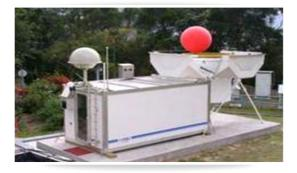
The Upper Air Sounding Sys (UASS) is a Meteorological equipment used to measure upper atmospheric weather parameters viz, Pressure, Temperature, Humidity, Wind Speed and Wind Direction at various heights with an aim to undertake aviation weather forecasting, missile firing and in identification of atmospheric ducts which is essential for establishing enhanced radar/sensorranges.
