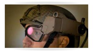
The Augmented Reality Head Mounted Display System is conceived as a capability enhancement to Land Based Air Defence Weapon Systems such as IGLA shoulder fired IR Homing AD Missile System and ZU 23mm 2B AD Gun System by providing
