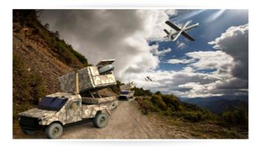
The MRPKS is proposed to be an indigenous Loitering Munition System to be developed and mounted on a vehicle. The launcher vehicle should have an integrated Launch Mechanism, Control Station, Communication Systems and Power Supply System. The munition should have a minimum range of 40 kms with an accuracy of less than 5 meters. The munition should have the capability to loiter in the target area for
